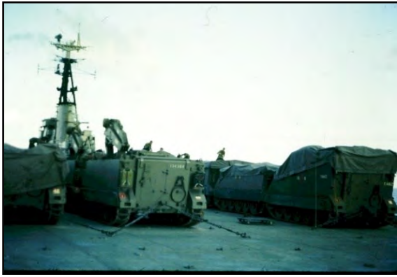
APCs secured on flight deck aft
